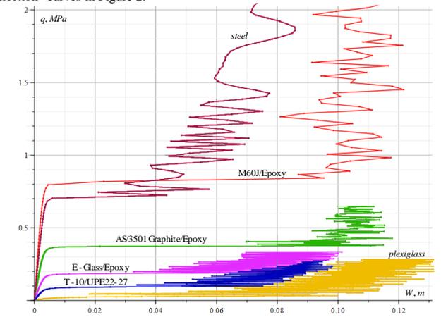
FIGURE 2. The "load-deflection" relations for the considered variants of shells
