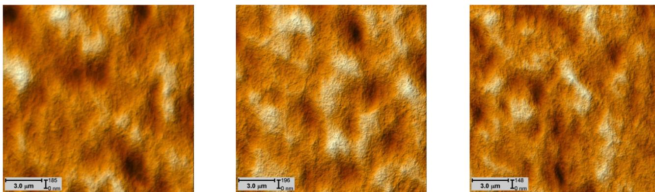
Stretched to 50% treated (0.1, 0.3 and 0.5 keV) surfaces. Axis of deformation is vertical.
