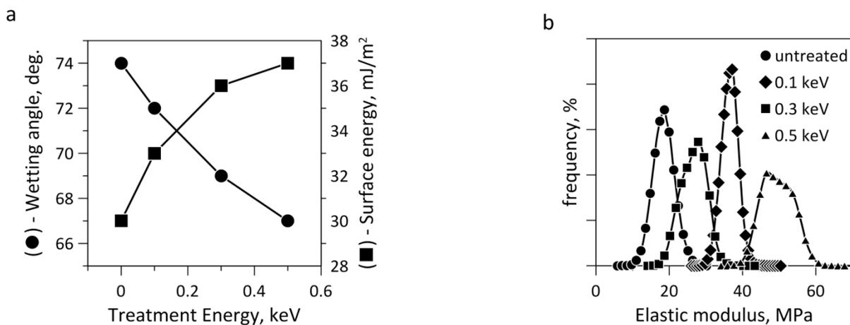
Wettability, surface energy (a) and elastic modulus (b) of the surfaces.
