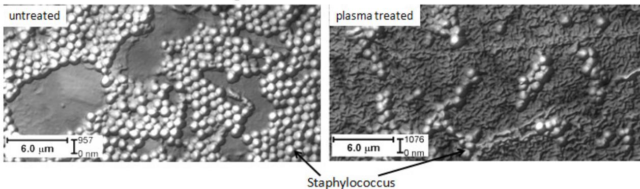
**The problem! Such coatings damage under deformation. The defects are the new centers of the bacterial growth.**
