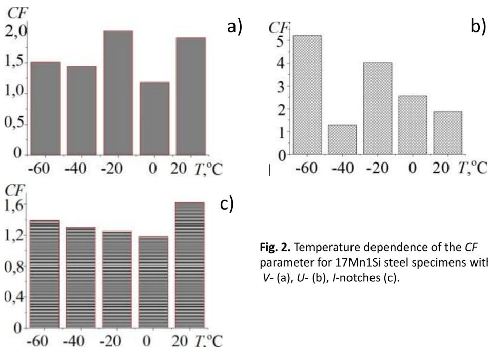
Fig. 2. Temperature dependence of the CF parameter for 17Mn1Si steel specimens with V- (a), U- (b), I-notches (c).
