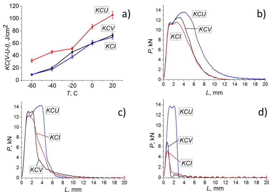
Fig. 1. Temperature dependence of impact toughness (a); impact diagrams in the load/displacement coordinates at test temperatures: 20 °C (b); –20 °C (c); –60 °C (d); for V-, U-, and I-notched specimens.
