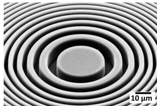
X-ray circular Fresnel Zone Plate from silicon manufactured by MEMS technology
