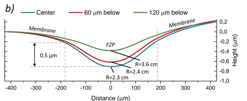
(a) Contour map obtained by the summation of the stereo images. (b) The horizontal deformation profiles of the FZP reconstructed at the different positions. The inflection points of the central profile are marked by A and B.
