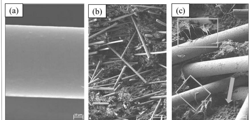
Fig. 3. Basalt fiber surface morphology and supramolecular structure of composites based on PTFE: (a) BF (x5.00k); (b) PTFE + 18 wt.% BF (x150); (c) PTFE + 18 wt.% BF (x500)
