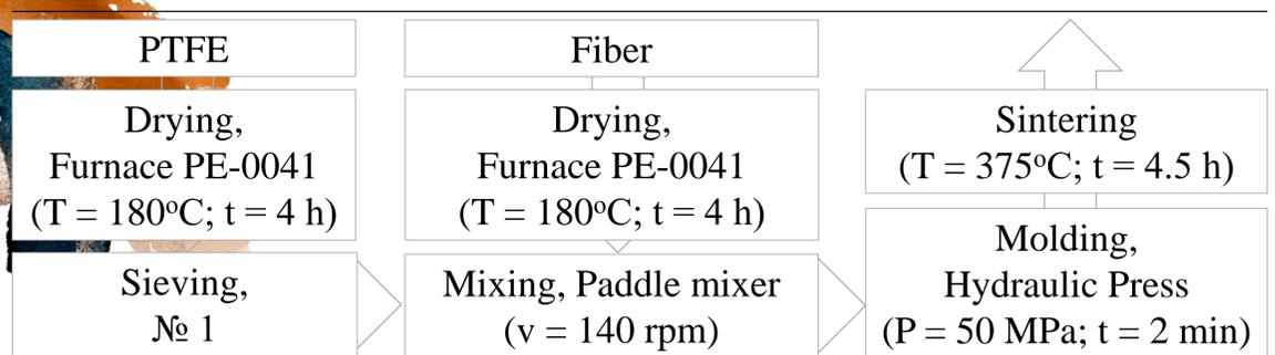
Fig. 1. Technological scheme for obtaining polymer composites based on PTFE
