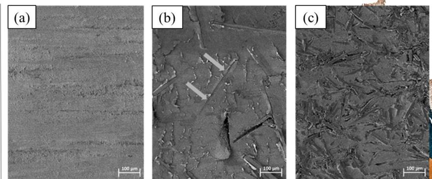
Fig. 2. Micrographs of friction surfaces of PTFE and its composites (x150): (a) PTFE; (b) PTFE + 18 wt.% BF; (c) PTFE + 18 wt.% CF
