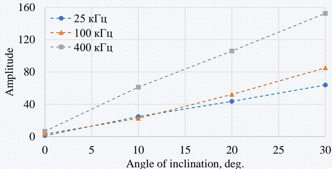
Pic. 8 – Dependence of the amplitude on the angle of inclination of the transducer
