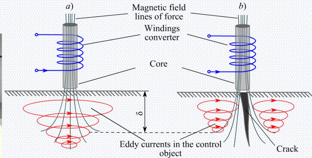
Рис. 4 – Schematic diagram of eddy current control
