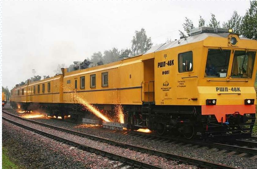
Pic. 2 – Rail grinding train operation
