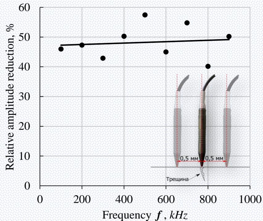
Рис. 6 – Dependence of the amplitude of the converter signal on the frequency of the excitation current on one crack
