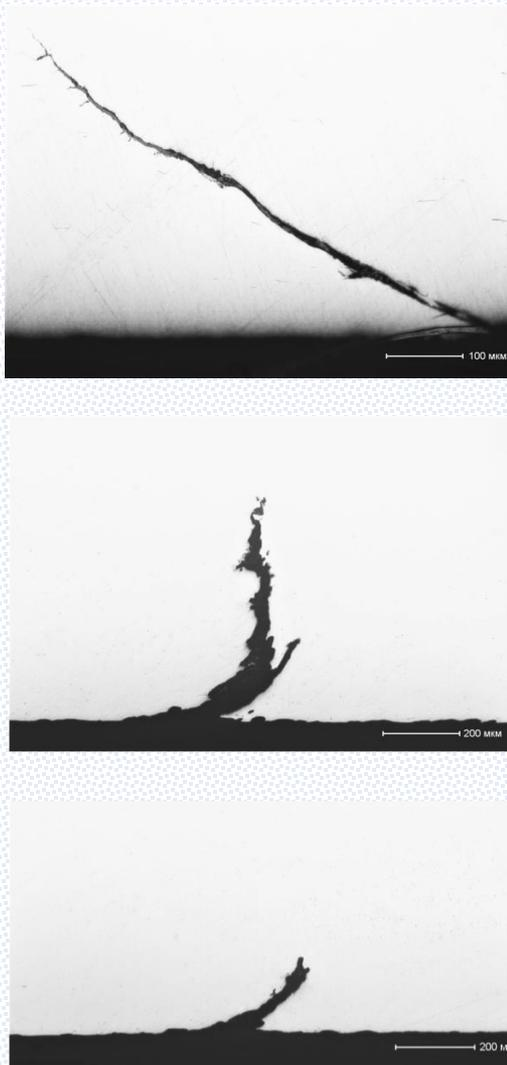
Fig. 12 – Photos of grinds with cracks
