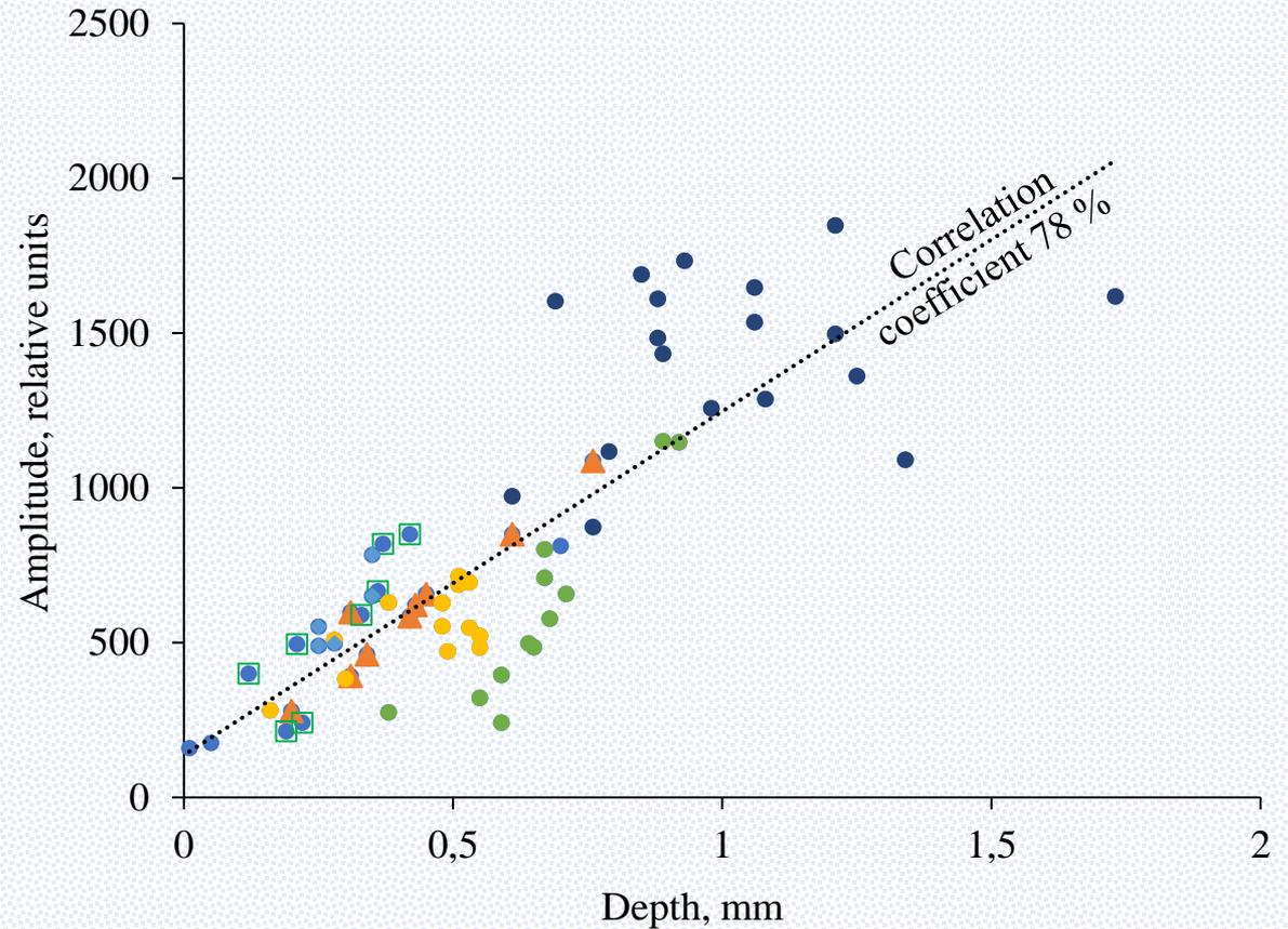
Fig. 13 – Dependence of the amplitude of the eddy current flaw detector on the depth of cracks for three samples
