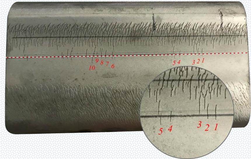
Pic. 11 – Marking of the sample with identified cracks
