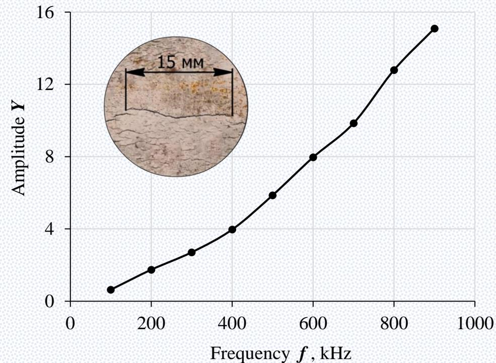
Pic. 5 – Dependence of the amplitude of the converter signal on the frequency of the excitation current at one crack
