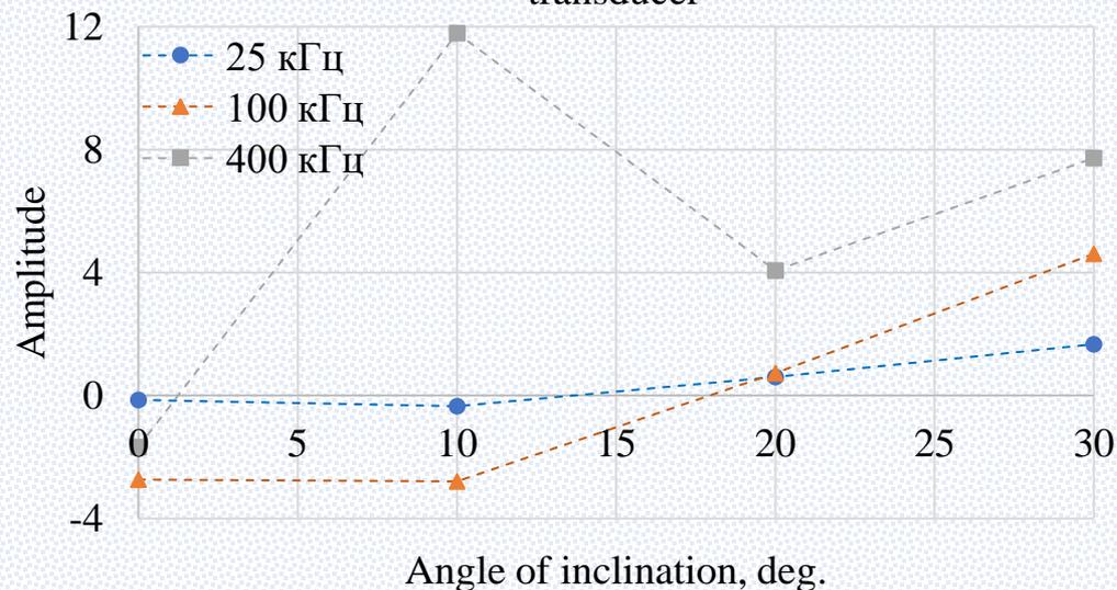
Pic. 9 – Dependence of the projection of the amplitude on the selected direction on the angle of inclination of the transducer
