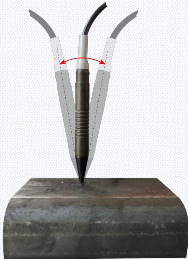
Pic. 7 – Tilt of the converter relative to the vertical axis
