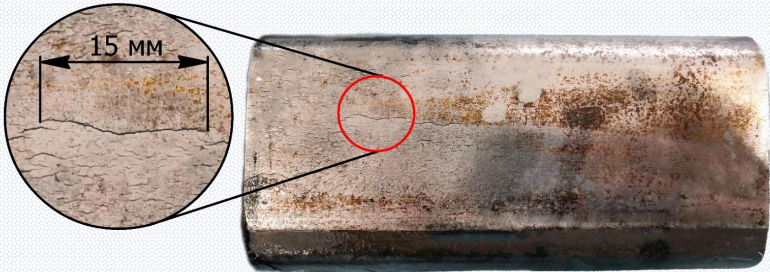
Pic. 1 – The rolling surface of the rail with contact fatigue cracks
